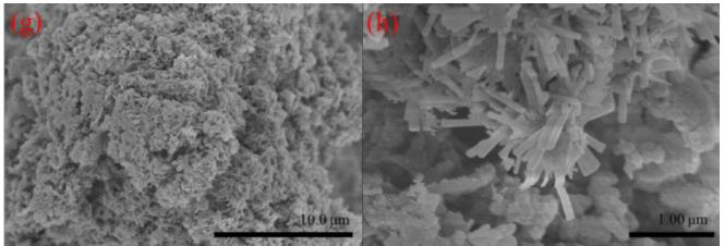
An electron microscope image of the kapok paper with microscopic deposits of zinc oxide and polyaniline.
